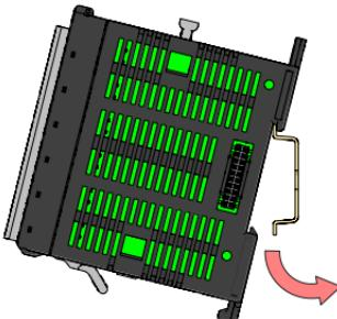
Rotate module ensuring clip snaps onto rail.
