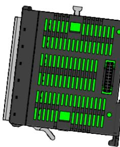
Insert DIN rail in mounting slots.
