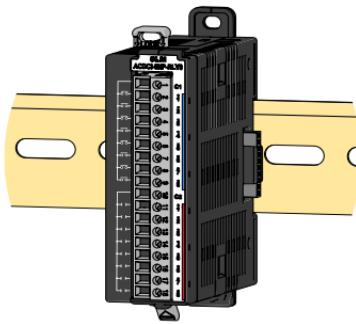
Module securely mounted on DIN rail.
