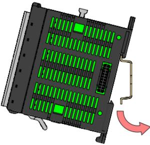
Rotate module ensuring clip snaps onto rail.
