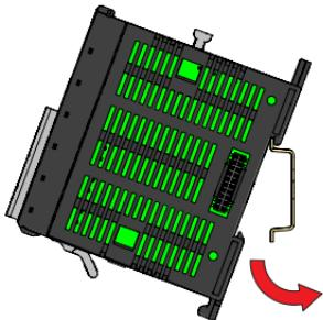
Rotate module ensuring clip snaps onto rail.
