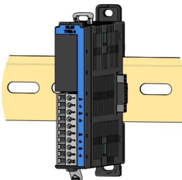
Module securely mounted on DIN rail.
