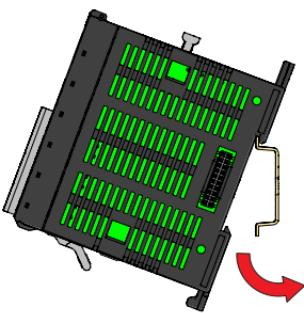
Rotate module ensuring clip snaps onto rail.
