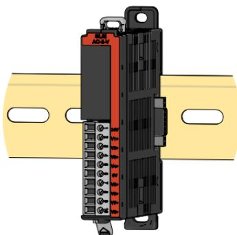
Module securely mounted on DIN rail.
